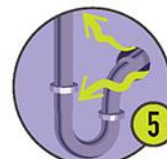
5 Gaps around service pipes
