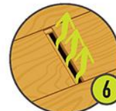
6 Gaps in suspended floors
