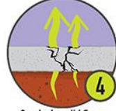
4 Cracks in solid floors
